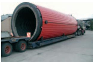
Thermal oil heater fired with sanderdust and/or natural gas with a capacity of 16 MW
